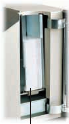
Large, 250-card input hopper requires fewer refills to keep production humming along.
